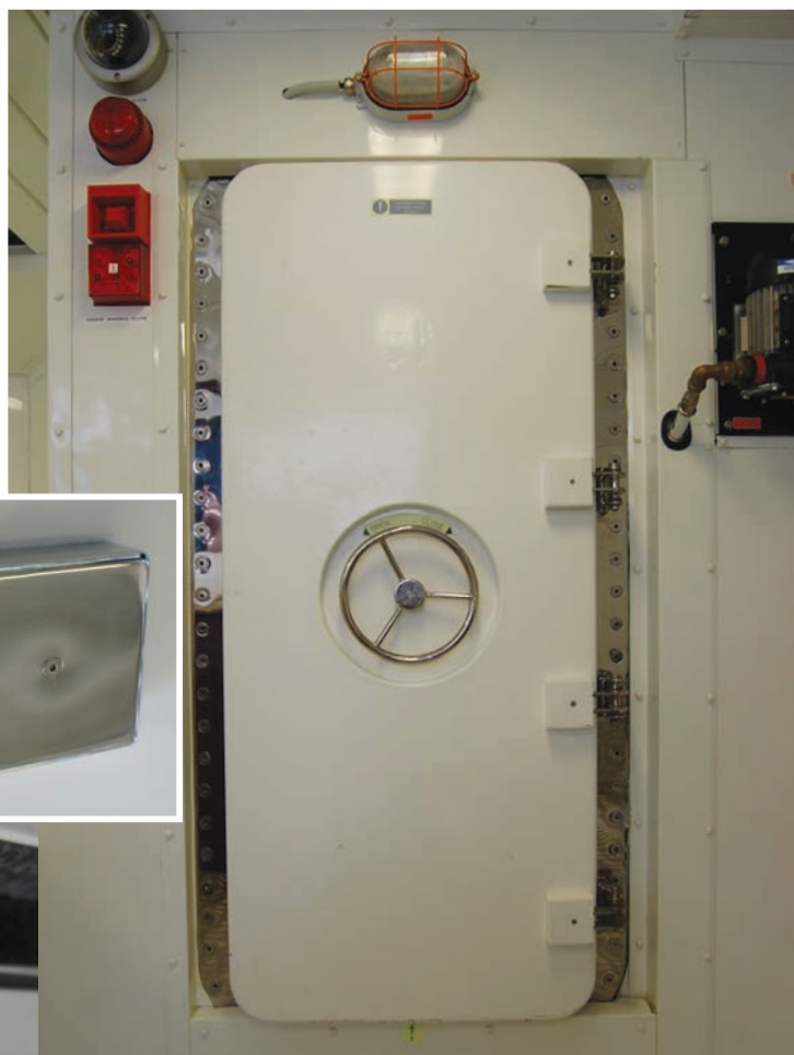
8 spade in acciaio inox 316 8 stainless steel Aisi 316 dogs
